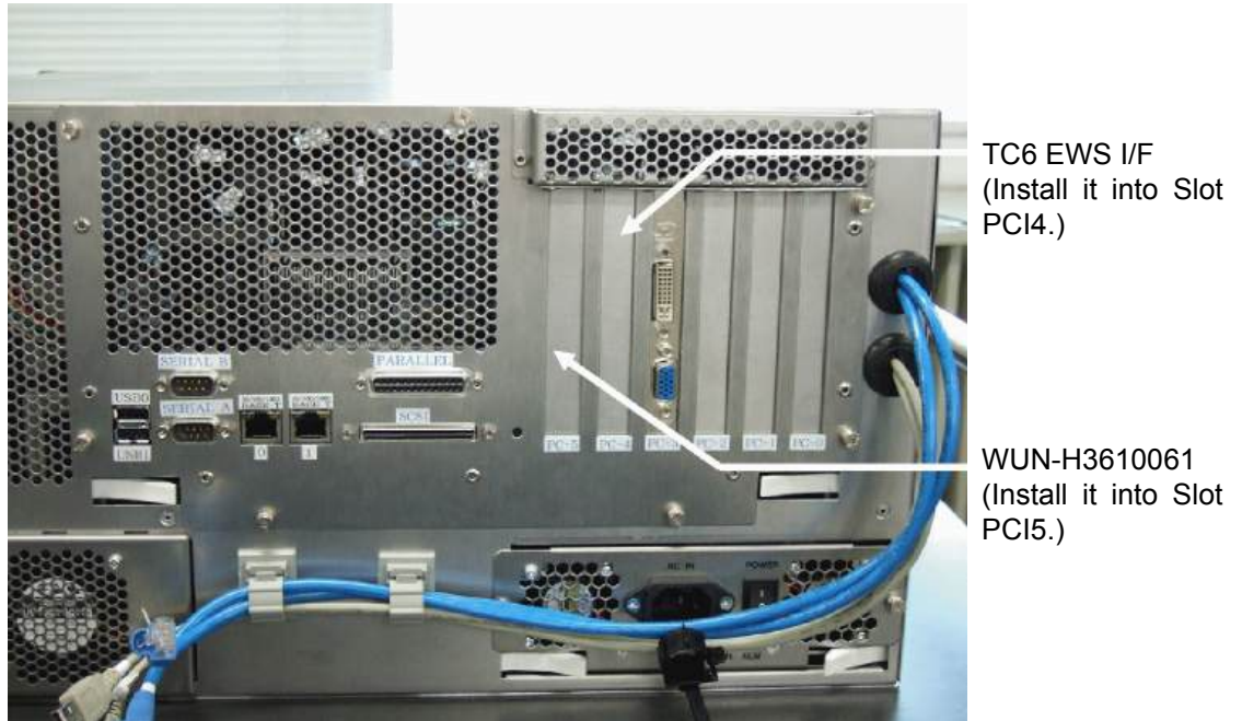
TC7A CPU Unit rear view
